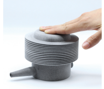
Figure 6: Bellow being pressed
