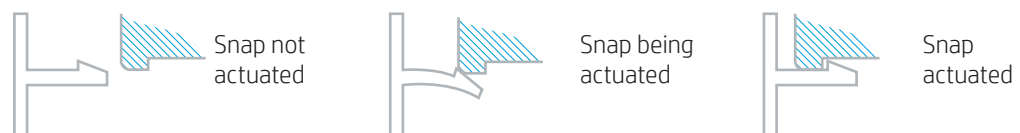
Figure 2. Cantilever snap-fit assembly operation
