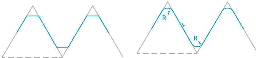
Figure 5: Round edges for custom-printed threads
