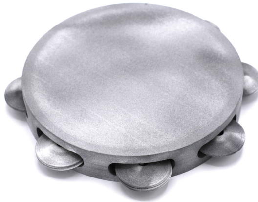
Figure 3: You can also 3D print percussive membranes, like the tambourine pictured above. Printing the tambourine with the membrane side down at a 30-degree angle helps avoid warpage of the membrane
