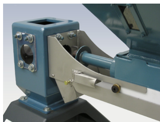
Auger assembly in calibration mode is ready to deliver catch samples of additive.
