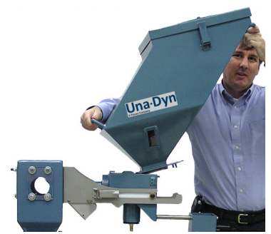
Grasp handles and slide material feed bin towards you and lift off.
