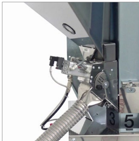
Quick discharge for the complete emptying of the residence hoppers
