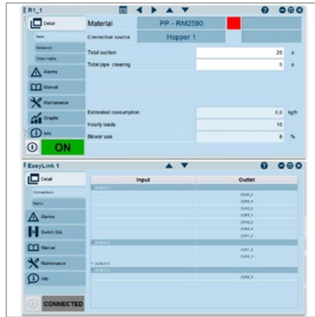
Material database, sources, destination matrix and line recipes can be easily created in WF4.0 and use for the automatic setting of Easylink+
