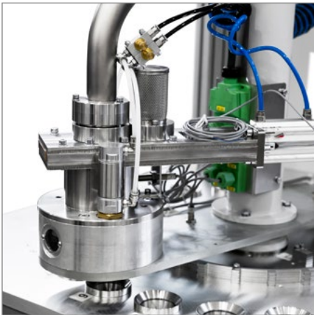
The internal arm is equipped with a local cleaning device, in order to avoid risk of contamination in the common part of the circuit
