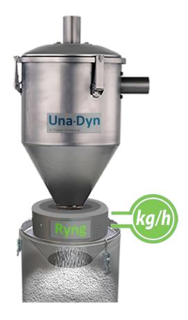
The Ryng is easy to install. The low-profile device is placed between the vacuum receiver and loaded vessel in order to weigh the amount of resin per load. The unit also totalizes the amount of resin used per selected time frame for data collection.
