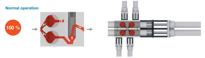
The heated steel housing allows for two screen bearing pistons, which contain two screen cavities each per piston. The melt flow is subdivided into four flow paths and is directed through each of the four screen cavities. Ongoing filtering leads to a rise in the resistance of the flow rate. When a defined pressure limit is reached, the screens are automatically cleaned by backflushing.
