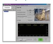
F.A.C.S. permits control of material conveying systems as well as monitoring of Maguire blenders, silo inventory, and most SPI compatible equipment such as dryers, mold temperature control units and chillers. The two-wire power and
